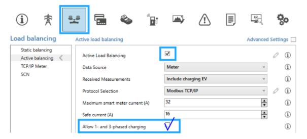
**Note:** the checkbox for 'Allow 1- and 3-phased charging'. This option must be active to allow an Energy Management System to control switching between single-phase and three-phases while charging. In the current implementation this option <u>must</u> be checked locally using the Service Installer Application.
