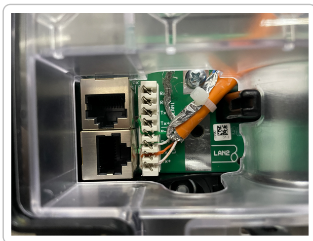
Figure 3. Connection LAN 2 Port via LSA+ terminal (HW3.0)
